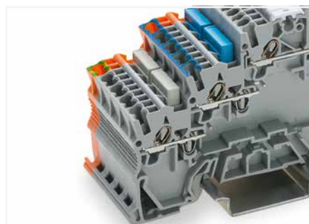
Ground commoning: For sensor and actuator terminal blocks without ground connection to the DIN-rail, the ground connection can be performed by commoning to the terminal block with a ground foot.
