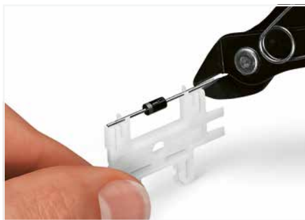
Cutting component to the proper length.
