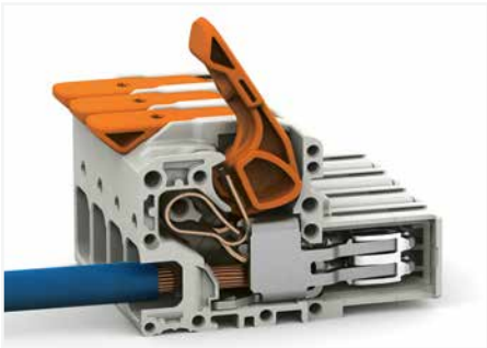
Insert fine-stranded conductors – and remove all conductors – via operating tool.
