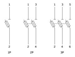
Wiring connection for devices with blown fuse indication
