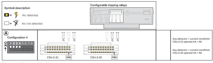
DIP switches 1, 2, 3 and 4 to position ON
