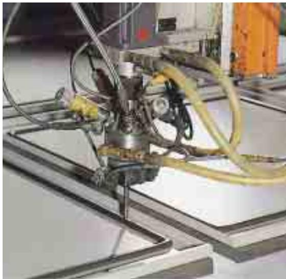
Polyurethane foam seal is applied to the door by a robot.
