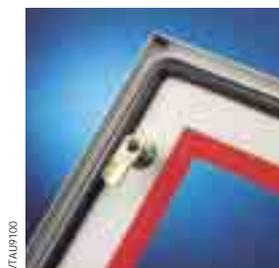
Steel plate doors (1.5 mm gauge). Application of polyurethane foam seal is robot-performed to obtain IP65 protection rating.
