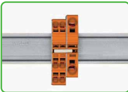
Commoning with push-in type jumper bars Commoning via open terminal side with end plate allows jumpering over two cross section sizes for 16 mm 2 /AWG 6 and 10 mm 2 /AWG 8 and one cross section size for 6/4/2.5 mm 2 (AWG 10/12/14); e.g., from 16 mm 2 /AWG 6 to 6 mm 2 /AWG 10 (see illustration above) or from 10 mm 2 /AWG 8 to 4 mm 2 /AWG 12.
