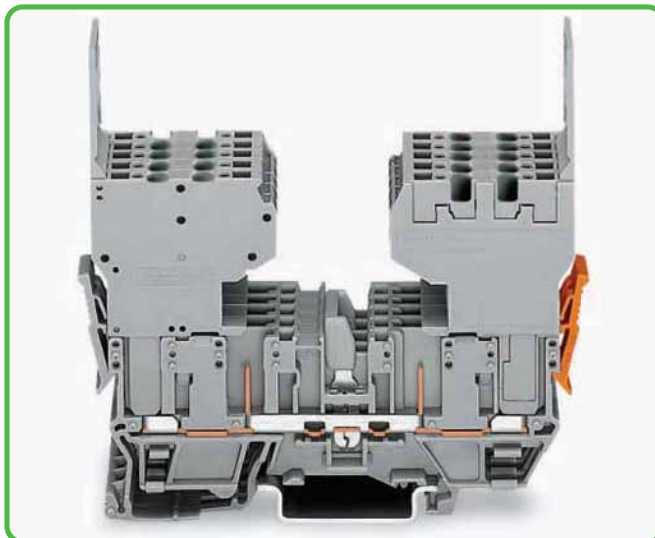
2 x 2-conductor female plugs - Commoning carrier terminal blocks via 280 and 780 Series jumpers and testing using 280-4.. test plug adapter.
