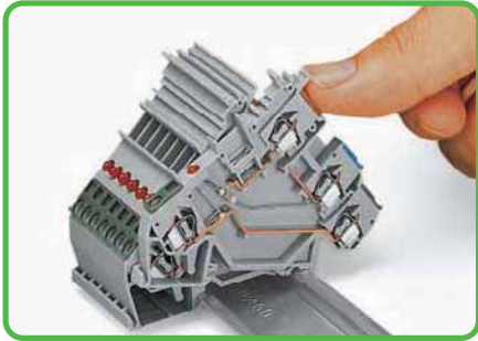
Assembly on the carrier rail. Terminal blocks with ground connection automatically establish a direct contact to the rail.
