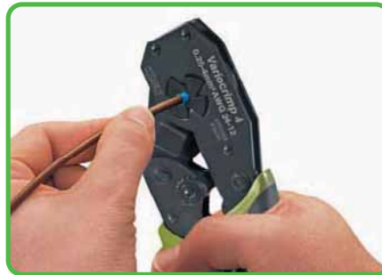
Squeeze handles until ratchet mechanism is released.
