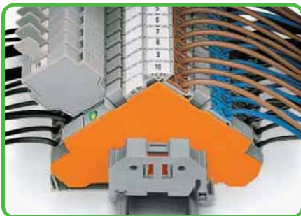
The fuse plug is 1 mm/0.039 in wider than the terminal block. This means an intermediate plate has to be fitted.
