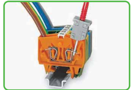
Testing via CAGE CLAMP® connection on the current bar - max. nominal current 6A; CAGE CLAMP® clamps individual test contacts.
