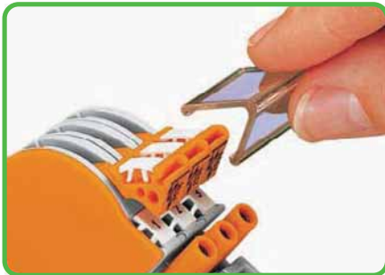
Transparent locking cover for 1 - 4 disconnect links can be snapped on a) for mechanical interlocking for multipole switching b) for protecting markers.
