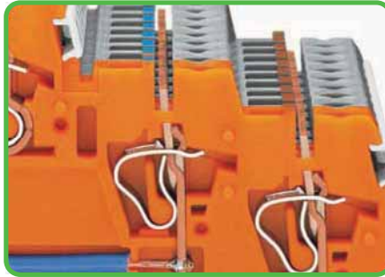
Commoning a supply voltage using uninsulated push-in type jumper bars, 2- to 9-way or 17-way (2 x 8 bits), depending on application.
