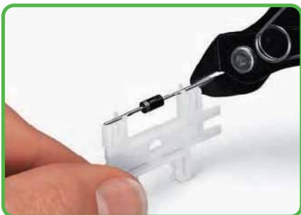
Cutting component to the proper length.
