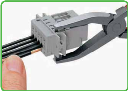
Conductor termination with operating tool (example shows a male connector).
