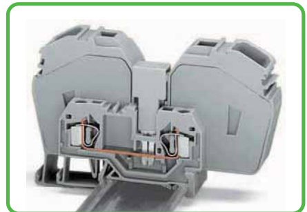
The 283-414 step-down jumper can even common 35 mm 2 (AWG 2) 285-635 through terminal blocks with 4 mm 2 (AWG 12) 281-901 through terminal blocks. For 35 mm 2 /AWG 12 through terminal blocks, see page 176.
