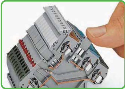
Commoning with adjacent jumpers. Push down the adjacent jumper until fully inserted.
