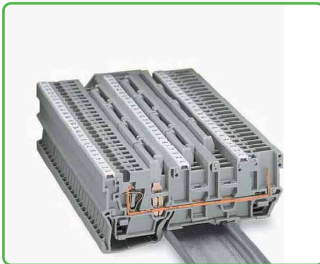
1-conductor/1-pin carrier terminal blocks with 3 jumper positions The 3 jumper positions allow up to six jumpering possibilities for staggered jumpers.
