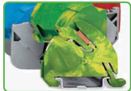
Carrier including a receptacle with locking device for 10 x 3 mm busbar. Contact between the busbar and rail is made automatically by simply snapping the carrier onto the DIN 35 rail. One end of the busbar is mounted onto the ground busbar carrier, the other end is inserted into the middle position of the insulated busbar carrier.
