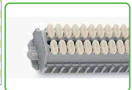
Terminal strip with fixing flanges, with push-buttons on one or both sides of the strip, for screw or similar mounting types, fixing hole 3.2 mm Ø (with 209-123 mounting adapter also for DIN 35 rail)
