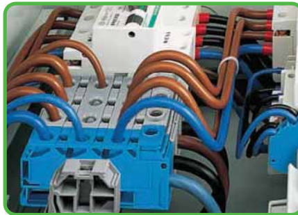
Rail-mounted distribution terminal block with 35 mm 2 /AWG 2 screw clamp connection (front-entry) and 3 x 10 mm 2 /AWG 8 front-entry CAGE CLAMP® connection.
