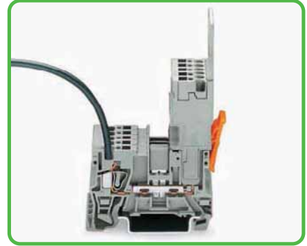
1-conductor/1-pin carrier terminal block: 769-176 Conductor cross section: 4 mm 2 /AWG 12
