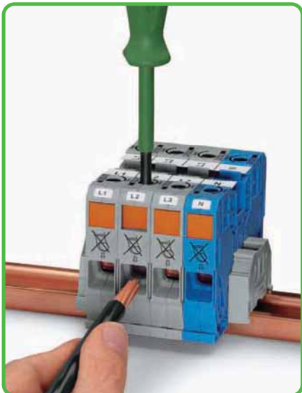
Insert stripped conductor into the clamping unit until it hits backstop; hold conductor in position.
