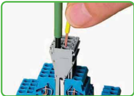
Tap-off modules are used when additional or removable connections are required (can be used as a permanent connection or a test plug). Wiring is possible whether the modules are plugged into the assembly or not.
