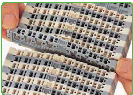
Slide terminal block and remove from the rail with a levering action.
