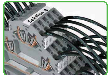
Marking clamping units with WMB Multi marking system (see Section 13). Group marking with 709-177 marker strips.
