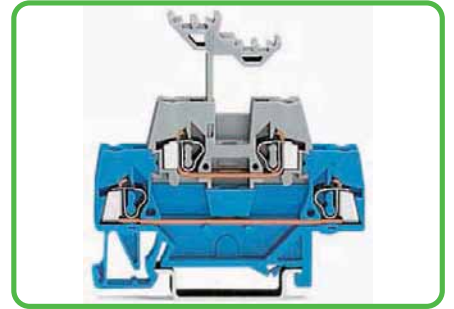
Double-deck terminal blocks accommodate two circuits of different potentials in one 2-level terminal block; different circuits can be differentiated by color coding either level for the 280 Series. The lower deck is wider than the upper, for ease of wiring.
