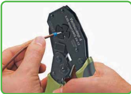
Insert ferruled conductor into crimping station.
