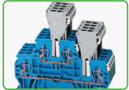
The module assembly can be directly inserted into jumper contact slots of the terminal blocks. The terminal blocks can also be commoned via push-in type jumper bars parallel to the jumper slots being used by the modules.
