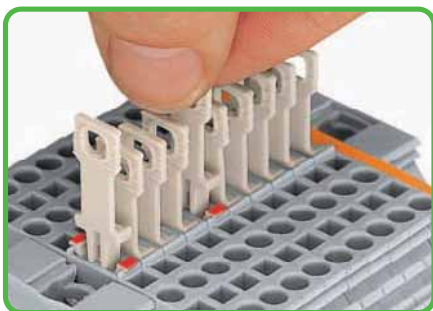
Pulling the disconnect tab by hand.
