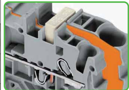
Commoning with step-down jumpers An end plate must be inserted between the terminal blocks to be jumpered. Step-down jumper 2006-499 commons 6/4 mm 2 (AWG 10/12) terminal blocks with 4/2.5/1.5 mm 2 (AWG 12/14/16) terminal blocks. Step-down jumpers are simply pushed down for full insertion, similar to other push-in type jumper bars.
