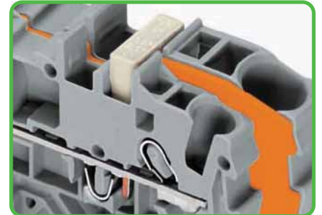
Commoning with step-down jumpers An end plate must be inserted between the terminal blocks to be jumpered. Step-down jumper 2006-499 commons 16/10 mm 2 (AWG 16/8) terminal blocks with 10/6/4/2.5 mm 2 (AWG 8/10/12/14) terminal blocks. Step-down jumpers are simply pushed down for full insertion, similar to other push-in type jumper bars.
