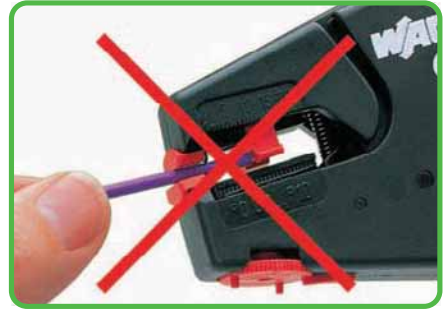
FIT CLAMP® terminations do not require stripping.
