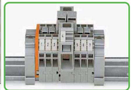
Commoning from 16 mm 2 /AWG 6 (283 Series) to 4 mm 2 /AWG 12 (281 Series) rail-mount terminal blocks.
