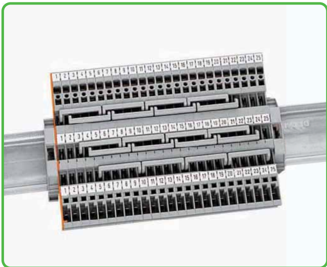
1-conductor/1-pin carrier terminal blocks with 3 jumper positions The 3 jumper positions allow up to six jumpering possibilities for staggered jumpers.
