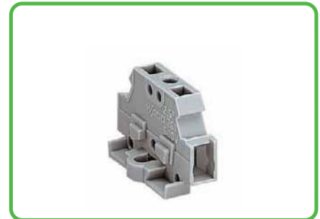
Terminal block with fixing flange, for screw or similar mounting types, fixing hole 3.2 mm Ø (with 209-123 mounting adapter also for DIN 35 rail) Lateral marking facility for miniature WSB Quick marking system, test slot.
