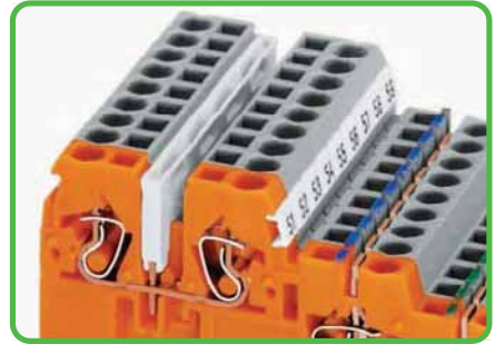
Commoning signal level voltage via insulated 870 Series push-in type jumper bars, 2- to 9-way, depending on application. Sensor LED terminal blocks cannot be commoned on the signal level.
