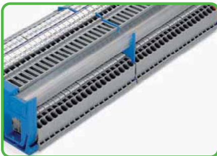
The compact busbar carrier, which is placed every 200 mm/7.87 in, provides additional busbar support for longer assemblies.
