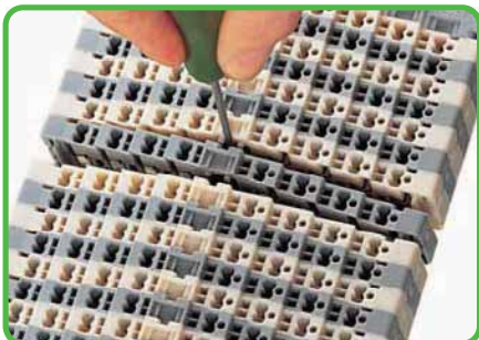
Open the assembly by laterally sliding a block via (2.5 x 0.4) mm operating tool.
