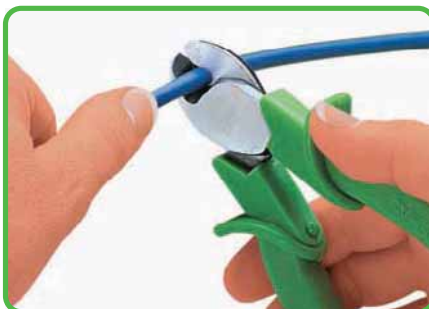
Cutting a conductor.
