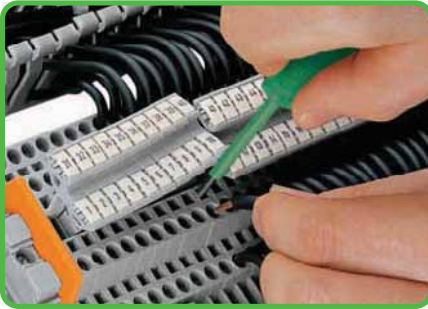
The flexible marker carrier, which is placed above the wiring level, can be pushed aside during wiring or comming. The marker carrier has two levels for two different markers relating to double-deck terminal blocks.
