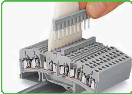
Used as potential multiplication. Inserting a 10-way, comb-style jumper bar (only possible in the center).
