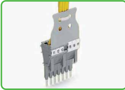
Module assembly with CAGE CLAMP® connections (0.25 mm 2 - 2.5 mm 2 /AWG 24 - 14), including strain relief plate and marker slots for miniature WSB or WMB markers.
