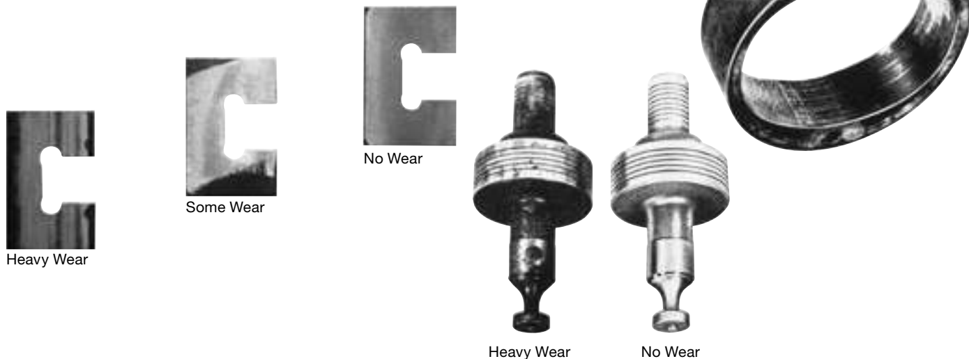
Figure 1. Typical Examples of Wear Due to Contamination
