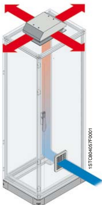
Natural aeration with hood (IP43) and grating.
